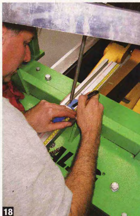
Dave made two reference marks on a piece of tape, one for where the steering head was and one for where it would need to go. In this case, just short of 7/10 inch. ►
